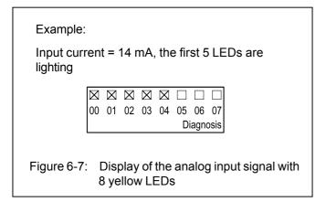
After pressing the test pushbutton for the first time, the channel E0 is selected: the related LEDs start flashing. After releasing the pushbutton, the analog value for channel E0 is displayed. The same process can be repeated for channels E1, E2 and E3.
